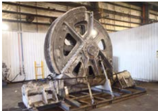
■ Before and after repair of a Fairlead Guide Roller with purpose designed delivery cradle.
