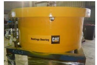
■ Rebuilt Lower Swing Pinion Housing Assembly
