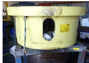
■ Rebuilt Lower Swing Pinion Housing Assembly
