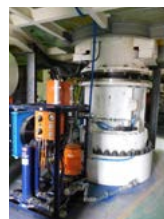
■ Original swing gear case and upgraded Planetary Swing Gear
