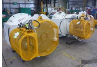
■ Before and after repair of a Fairlead Guide Roller with purpose designed delivery cradle.
