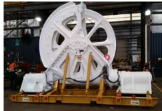
■ Before and after repair of a Fairlead Guide Roller with purpose designed delivery cradle.
